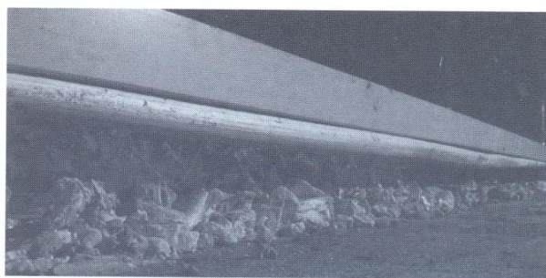
Fig. 8. A wych elm stave is simultaneously set straight as its belly is heat-tempered over embers.
