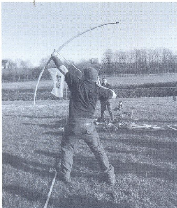
Fig. 12. A wych elm warbow that draws one hundred and thirty four pounds at full draw and would provide an excellent yew bow substitute whilst shooting at the butts or in battle. It measures only seventy inches from nock to nock yet has no compression frets. It is also, in the right hands and with ideal weather, capable of reaching bowshot with a replica Westminster Abbey arrow.
