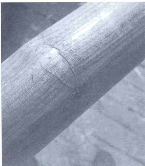
Fig. 2. A potentially catastrophic fret emanating from a pin on the belly of a 110lb rowan warbow.
